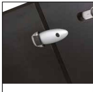
1 set consists of a male and a female part made of zamak. Fixation by means of 4 wood screws, a zamak screw-in bushing and a fifteen screw.
